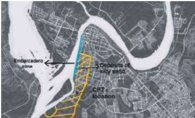
Figure 2: Location of CPTu soundings performed on silty soil deposit
