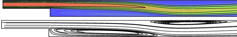
FIGURE 10. The backward facing step problem  $Re = 800$ . Isovalues  $|\mathbf{u}_h|$  (top) and the streamlines of the velocity (bottom) using the final adapted mesh (63.506 elements) with the  $\mathbb{P}_1^2 \times \mathbb{P}_0$  element.
