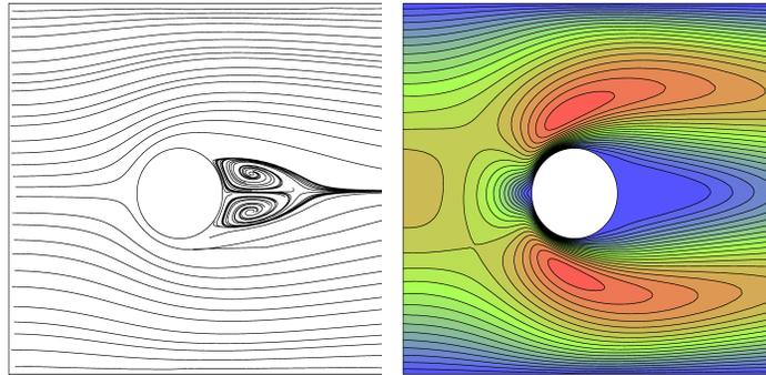
FIGURE 13. The circular cylinder problem with  $\nu = 10^{-3}$ . Zoom of the streamlines and the isolines of  $|\mathbf{u}_h|$  in the final adapted mesh for the  $\mathbb{P}_1^2 \times \mathbb{P}_1$  element (60.593 elements).
