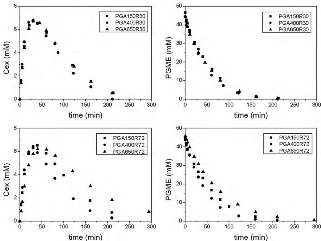
**Fig. 2.** Operation curves of batch reactor for the synthesis of Cex with biocatalysts of different sizes (R30 and R72) and enzyme loads (150, 400 and 650 IU/g<sub>cat</sub>), showing Cex and PGME profiles.
