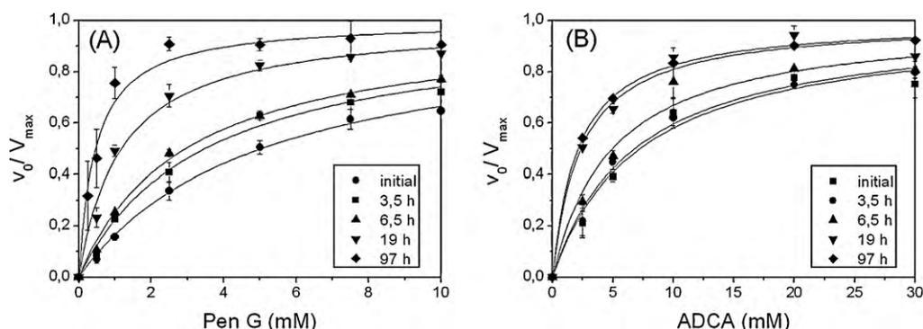
**Fig. 4.** (A) Normalized initial reaction rates of penicillin G (PenG) hydrolysis ( $v_0/V_{max}$ ) at varying PenG concentrations for mechanically ruptured PGA650R50 biocatalyst; (B) normalized initial reaction rates of cephalixin synthesis ( $v_0/V_{max}$ ) at varying ADCA concentrations and 100 mM PGME for mechanically ruptured PGA650R50 biocatalyst. Symbols correspond to data points; lines correspond to the respective fitted Michaelis–Menten equation.
