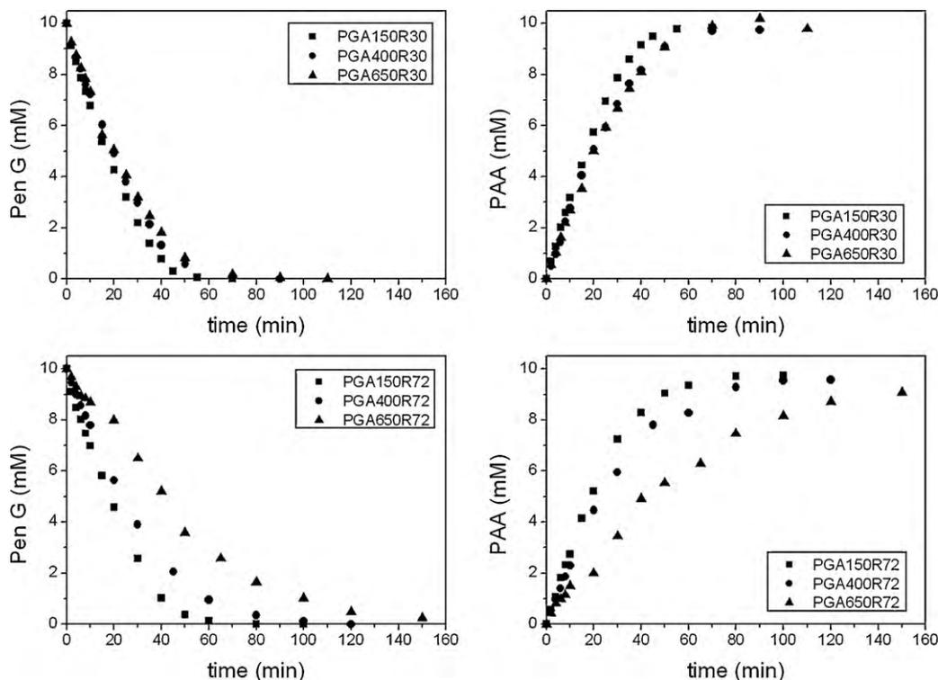
**Fig. 1.** Operation curves of batch reactor for the hydrolysis of penicillin G (PenG) with biocatalysts of different sizes (R30 and R72) and enzyme loads (150, 400 and 650 IU/g<sub>cat</sub>), showing PenG and PAA profiles.
