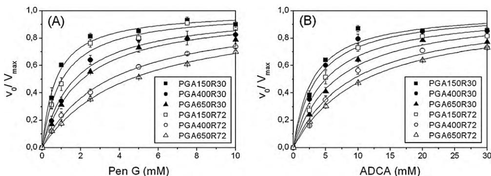
**Fig. 3.** (A) Normalized initial reaction rates of penicillin G (PenG) hydrolysis ( $v_0/V_{max}$ ) at varying PenG concentrations with PGA biocatalysts of different sizes and enzyme loads; (B) normalized initial reaction rates of cephalixin synthesis ( $v_0/V_{max}$ ) at varying ADCA concentrations and 100 mM PGME. Symbols correspond to data points; lines correspond to the respective fitted Michaelis–Menten equation.
